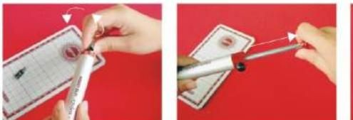
Screw the puncher or setter into the handle of the eyelet tool.
