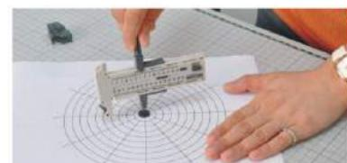
The blade can be replaced to the pencil lead and it can be used for drawing various circle.
