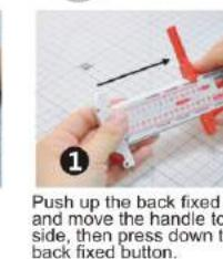
Move right the grip to the cutting size. And lock the fixator before using.
