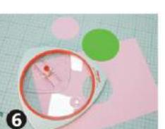
6 Finished. Tighten the control button to withdraw the blade.
